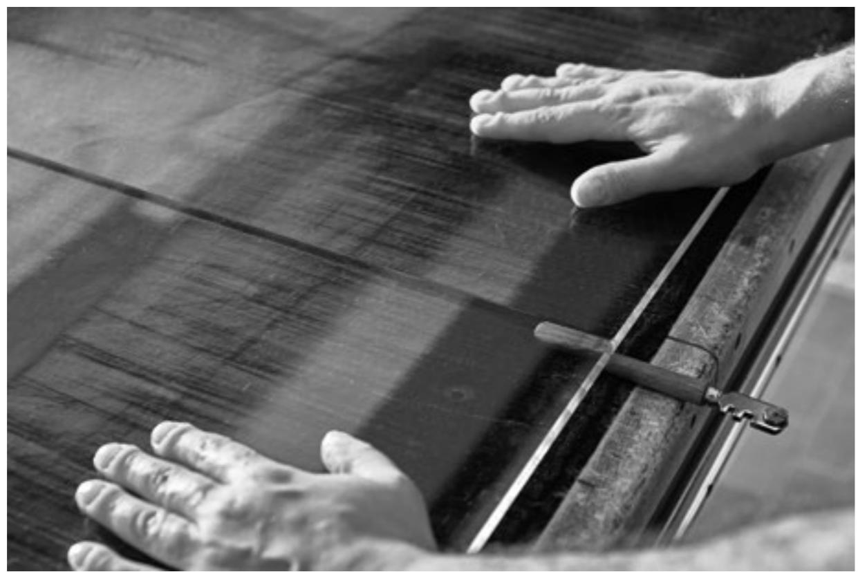
A particular type of grinding is the bevelling, a very delicate processing used above all for elements and mirrors of great value. Starting from the edge, a frame effect is created across the whole surface of the glass.
